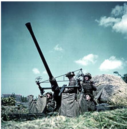
British 40mm L/60 includes the British-designed *Stiffkey Sight*, being operated by the gun layer standing on the right. The layer operates the trapeze seen above the sights, moving them to adjust for lead. The loader stands to the layer's left, and the two trainer/aimers are sitting on either side of the gun.
