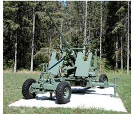
Q.F. 40 mm Mk. 1 displayed at CFB Borden. This example mounts a Stiffkey Sight, and displays the additional armor protecting the gunners.
