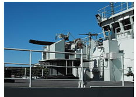
The L/60 Bofors fitted to the Kingston-class coastal defence vessel HMCS Nanaimo
