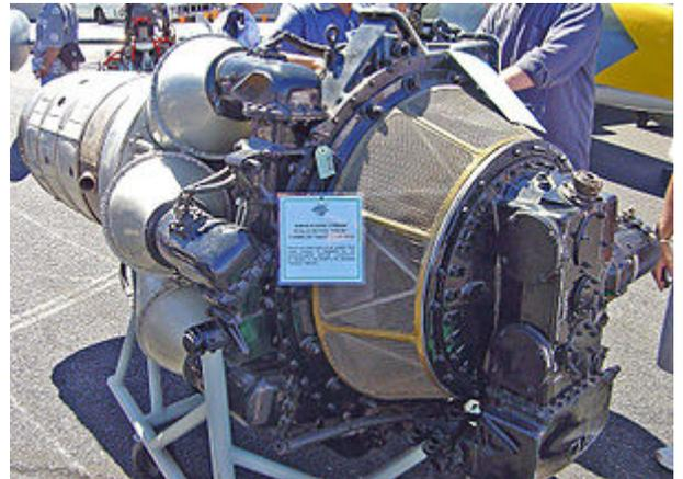
Rolls-Royce Nene on display at RAAF Base Pearce, Western Australia - note the wire mesh grille around the air intake to prevent Foreign object damage
