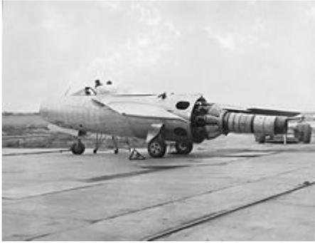
An FMA IAe 33 Pulqui II without tail section, showing its Rolls-Royce Nene II turbojet
