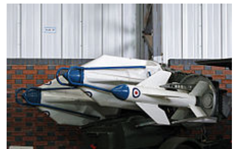
Tigercat three-missile launcher with inert training round (right) and transit covers in place
