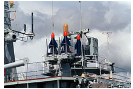
Seacat launcher and GWS-22 director on HMNZS Wellington , a Leander -class frigate. Notice the operator's CCTV camera on the director and the orange dome, housing the antenna for transmitting commands to the missile
