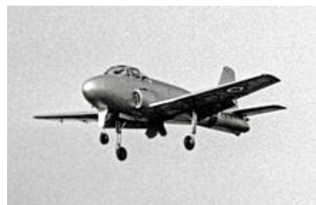
The prototype Jet Provost T.1 with the initial longer undercarriage at the Farnborough Air Show in 1954
