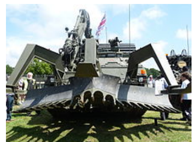
TROJAN AVRE with Full Width Mine Plough and Fascine.
