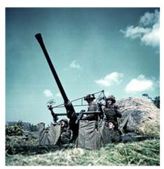
British 40mm L/60 includes the British-designed *Stiffkey Sight*, being operated by the gun layer standing on the right. The layer operates the trapeze seen above the sights, moving them to adjust for lead. The loader stands to the layer's left, and the two trainer/aimers are sitting on either side of the gun.
