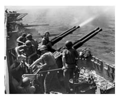
A MK 12 quadruple mount of Bofors guns fires from USS *Hornet*
