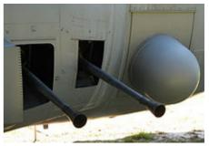
When four additional AC-130Us were to be converted from 2002, the necessary 40 mm L/60 guns had to be salvaged from old M42 targets at the Nellis AFB range.<sup>[21]</sup>
