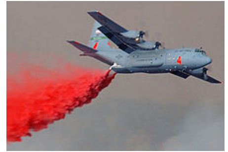
A C-130E fitted with a MAFFS-1 dropping fire retardant
