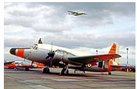
Valetta T.4 of No.2 ANS with extended radar nose
