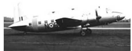
Vickers Valetta T.3 of the RAF College at Blackbushe airport in September 1956. Note the cabin-top astrodomes and aerials for navigational training
